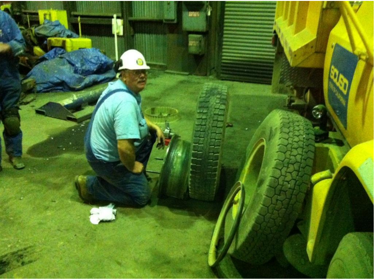
Chris works on changing the tire on the dump truck
